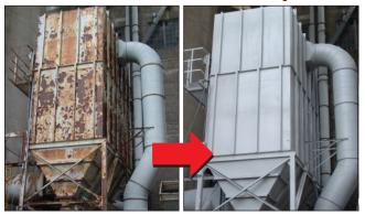
ENESEAL® CR is a single component, water based, liquid coating which dries to a highly durable, corrosion resistant, elastomeric 'skin' that provides extraordinary environmental protection to metal and concrete / masonry surfaces.
