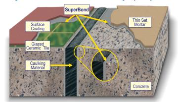
A revolutionary structural adhesive that provides unrivaled performance when bonding a new concrete overlay to an existing, cured concrete surface or when bonding synthetic / plastic mortars to virtually any rigid surface.
