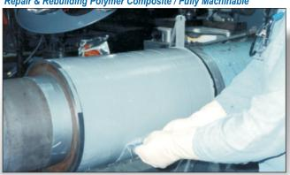
Multi-purpose; can be drilled, tapped, turned on a lathe, sanded and polished. Can be used to repair worn shafts, cracked casings and engine blocks, stripped threads, sloppy keyways, scored hydraulic rams, oversize bearing / bush housings, etc.
